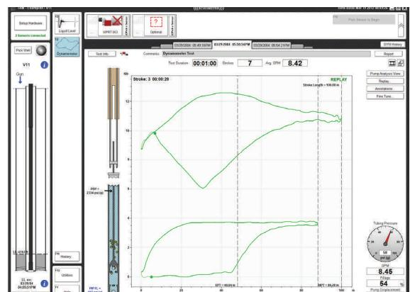
After two complete strokes the surface and pump dynamometer cards are displayed in real time. End Acquisition with the "Stop" button.
